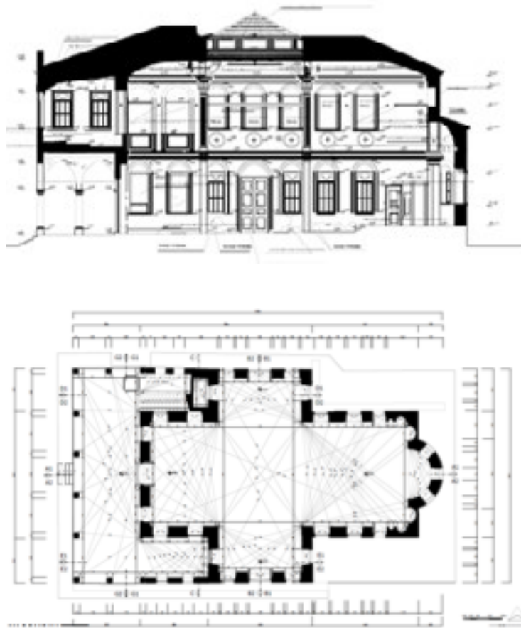
Figure 9. a) Section of Saint Voukolos Church b) Ground floor plan of the church [14]
